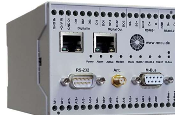
2x Ethernet-Interface for IT/OT separation
